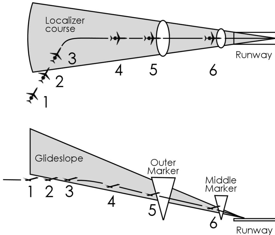
1. Tune the NAV radio to the desired localizer frequency and set the course arrow to the published inbound front course. Rotate the mode selector to N/L. If the aircraft is more than approximately 2 dots from the localizer centerline, the mode annunciator N-L ARM light will illuminate. Steering commands are still referenced to the heading marker which is set to the desired intercept heading.
