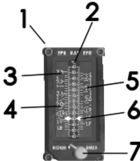
**1. RAM AIR TEMPERATURE/ENGINE PRESSURE RATIO (EPR) INDICATOR**
