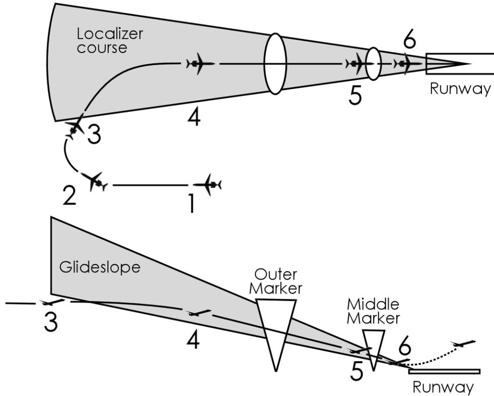
1. Tune the navigation radio to the desired ILS frequency. Set the inbound localizer course on the HSI. Turn the NAV SELECTOR switch to the ILS position. The mode annunciator displays N-L ARM and G-P ARM indicating the automatic pilot is armed for automatic beam capture.
