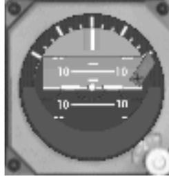
A gyroscopic standby attitude indicator is provided on the Captain's instrument panel.
