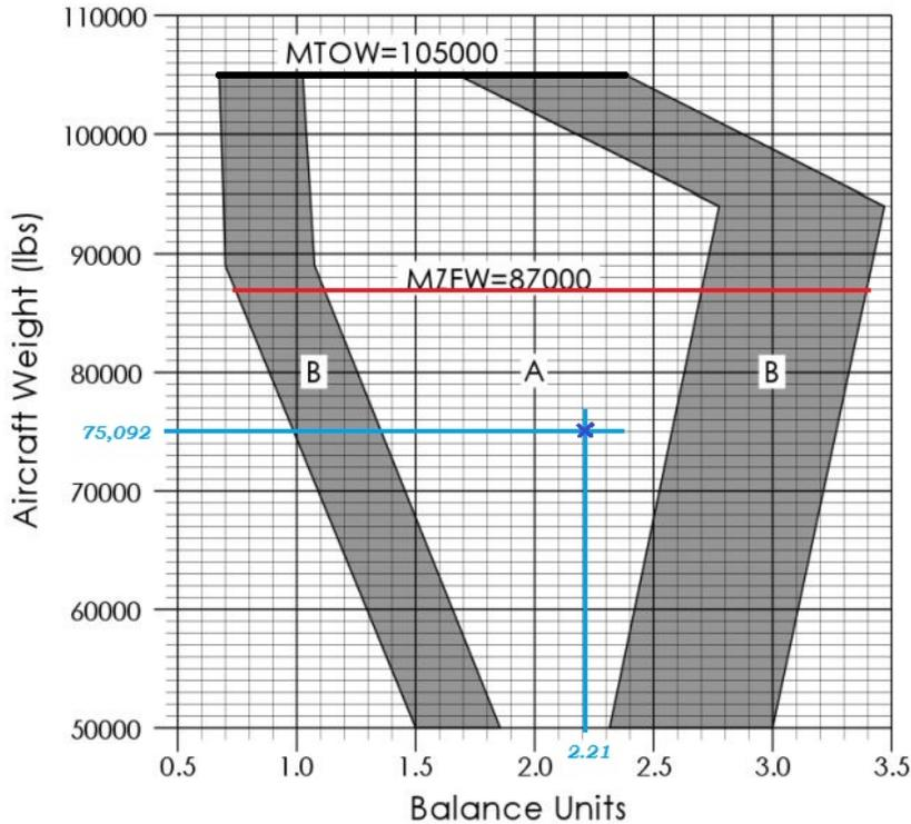
Once the values have been plotted on the Balance Graph and have been found to be legal, then a checkmark is placed in the box to the left of the ZFW value.
