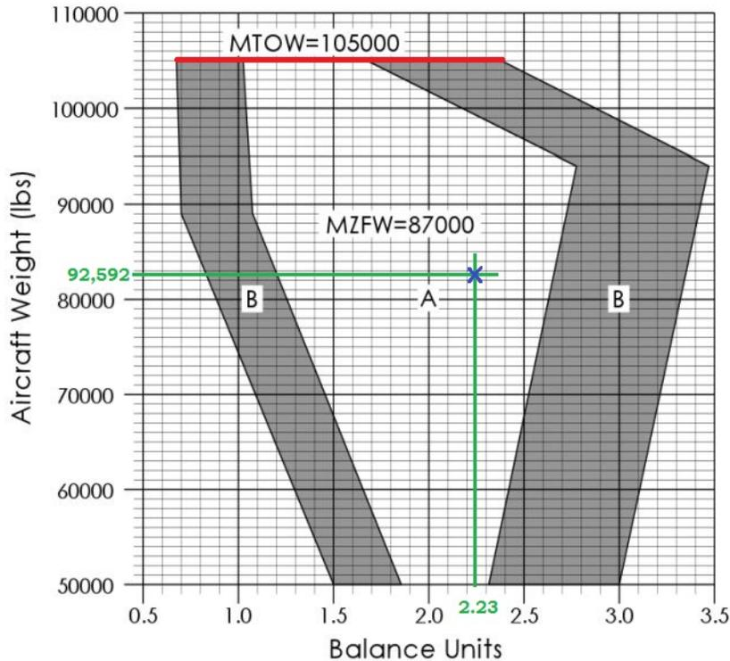
Again, the point clearly falls within area **A**. And it is well below the Maximum Takeoff Weight of 105,000 lbs. (A value which is so important that we wrote it earlier on the Weight and Balance Control form to make sure it would not be exceeded.) Once this has been verified on the graph, you should put a checkmark in the box on the **TAKEOFF GROSS WEIGHT** line.
