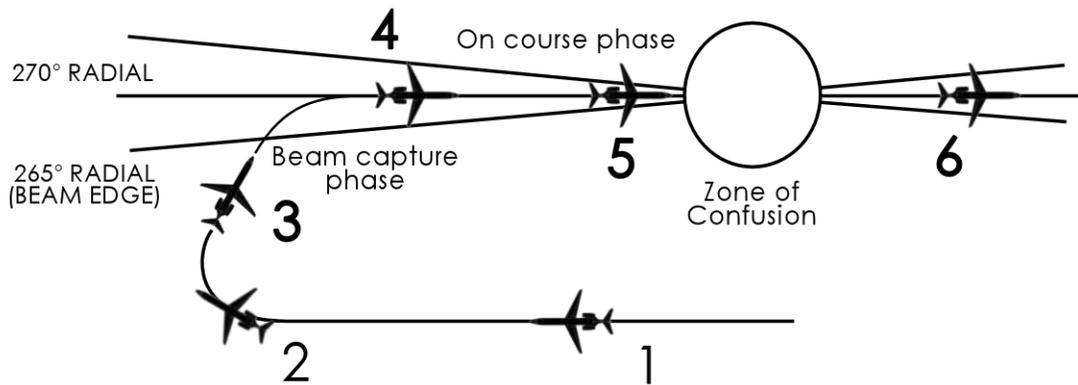
1. Tune the navigation radio to the desired VOR station frequency. Set the desired course on the HSI. The deviation bar on the HSI indicates your position relative to the desired VOR radial. Turn the NAV SELECTOR switch to the NAV LOC position. The mode annunciator displays N-L ARM to indicate the automatic pilot is armed for automatic beam capture.
